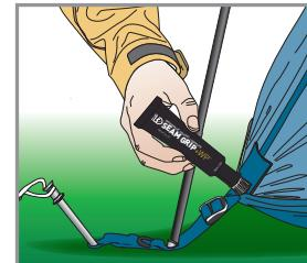
Apply Seam Grip+WP to the inside of the perimeter floor seam. This seam is not taped at the factory. Draw seam sealer across threads and under folds.
