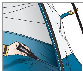
After years of service, seam tape on tents and outerwear can peel or pucker and the seam will begin to leak. If a small section has peeled use Seam Grip+WP to reattach it. If the tape seems to be failing everywhere, remove the tape and discard it, then clean the seams with Isopropyl
