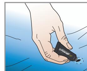
To ensure Seam Grip+WP does not run, apply a thin layer and when possible apply and allow to dry on a level surface area.
